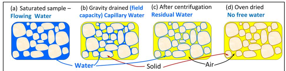
Schematic representation water state at the four extraction stages: (a) saturated, (b) at field capacity, (c) residual water after centrifugation, and (d) after oven drying (no water).
