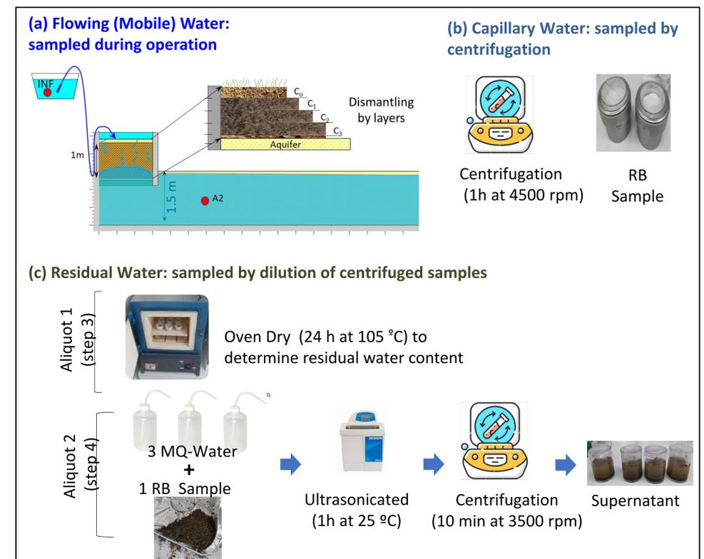
The image (a) Cross section of rbSAT sampled at INF (inflow) and A2 for flowing water during operation, the RB was dismantled by layers (C<sub>0</sub> through C<sub>3</sub>) after 1 day drainage; (b) extraction of the water retained by capillarity; and (c) extraction of residual water.
