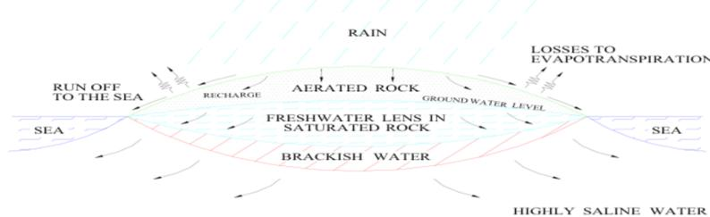
Diagram of a Freshwater Lens in an Oceanic Island (Like The Bahamas)
