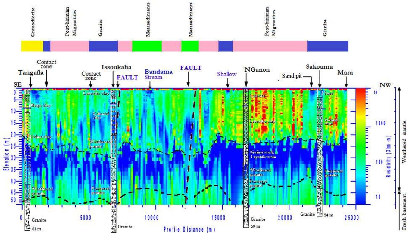
Figure 6 - 1D Resistivity section with geology settings, drilling logs, weathering profile, hydrogeology boundaries under large EM profile SE-NW on investigation area.
