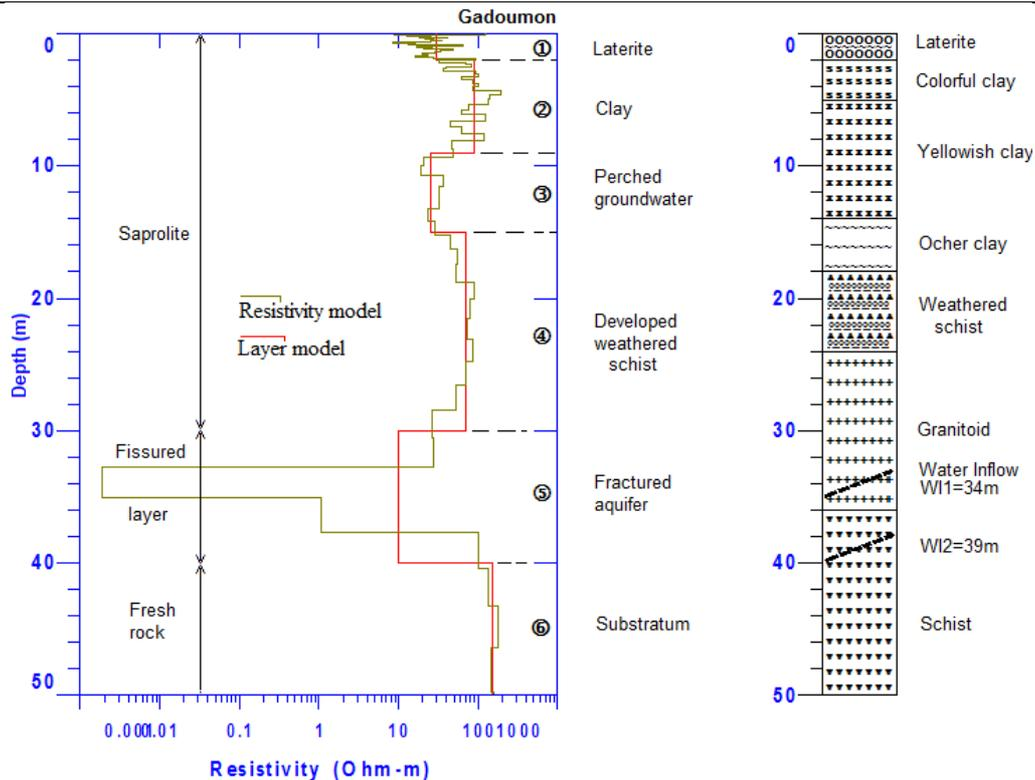
Figure 5 - 1D six-layer inversion model (resistivity/depth) from Gadoumon site, with well log
