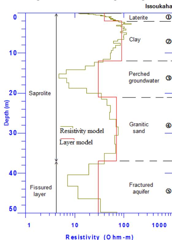
Figure 4 - 1D five-layer inversion model (resistivity/depth) from Issoukaha site
