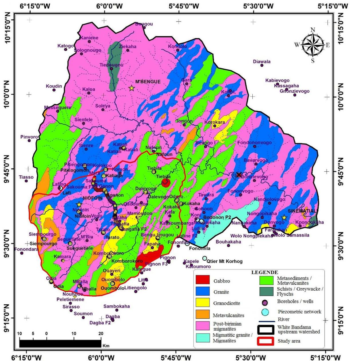
Figure 1 - Geological map of the White Bandama upstream watershed (simplified from Geomines, 1982) with location of survey area, observation wells, electromagnetic (EM) profile.
