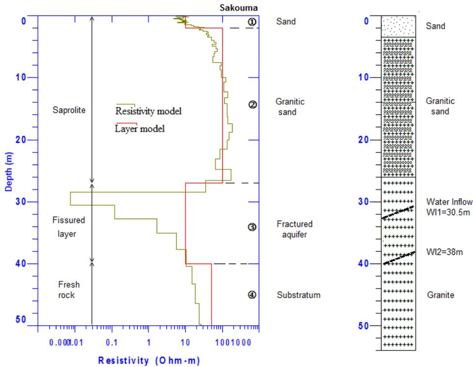
Figure 3 - 1D four-layer inversion model (resistivity/depth) from Sakouma site, with well log
