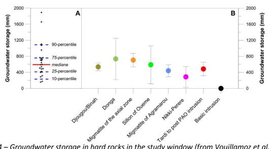
Figure 4 – Groundwater storage in hard rocks in the study window (from Vouillamoz et al., 2015). A: Percentile. B: Variation of storage among geological units (the point is the median value and the error bars are the mean difference to the median).
