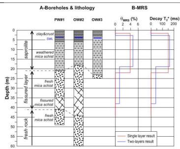
Figure 5 – Experiments at ARA site. A: Borehole lithology. SWL is the static water level. B: MRS results (modified from Vouillamoz et al., 2014).
