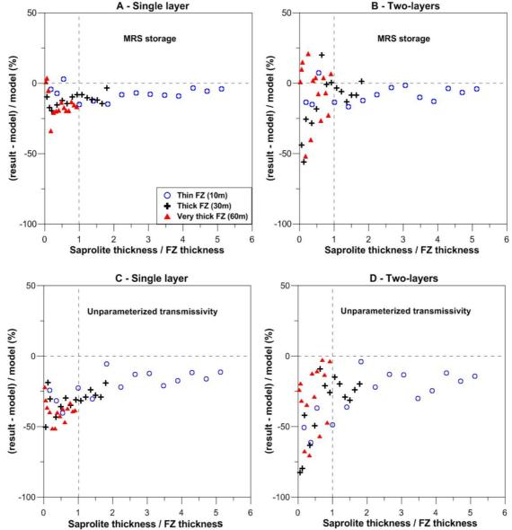
Figure 6 – Comparison of the MRS single and two-layer results to the initial model results. A&B: MRS storage. C&B: No-calibrated transmissivity.
